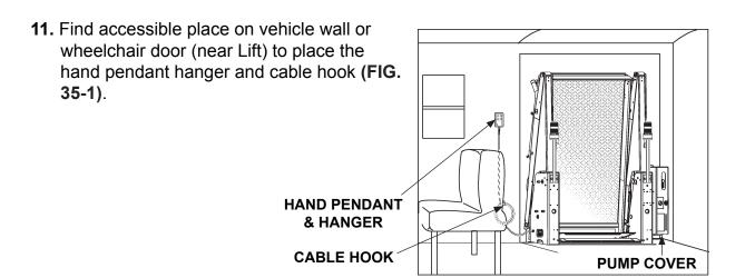
TYPICAL LOCATION (INSIDE VEHICLE) FOR STOWING HAND PENDANT FIG. 35-1
